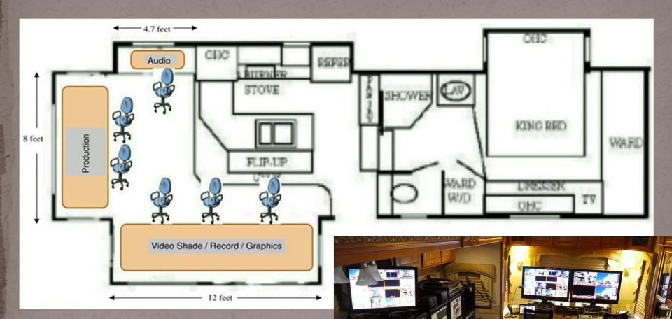
The trailers two production area slide outs offer an expanded work area, creating a very comfortable environment with many of the RV associated comforts, including an on board restroom. Accommodations available for EIC/Engineer, a possible budget resource.
