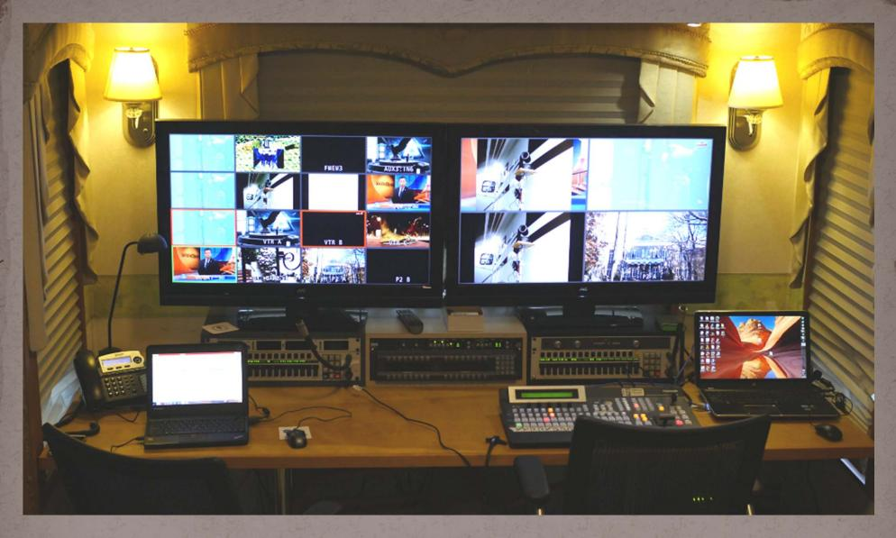
The production area features a Panasonic HS450N, 16+ Input HD Switcher with Dual-Screen Multi-viewer Display. The monitor wall can accommodate either a 9-4 or 16-4 display. Four AUX outputs with AUX 1 having dissolve transitions. 8 HD-SDI outputs, 4 outputs incorporating up/down conversion. Recently added 40x40 BMD 4K UHD video router with BMD 2ME 4K switcher and RTS Zeus III matrix intercom system.
